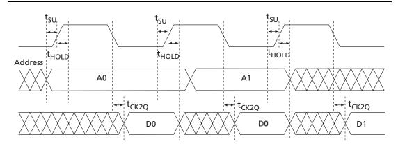
Figure 2-45 • FlashROM Timing Diagram
