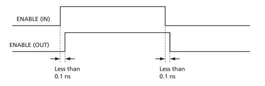
Figure 2-100 • Timing Diagram (option1: bypasses skew circuit)
