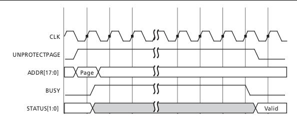
Figure 2-41 • FB Unprotected Page Waveform
