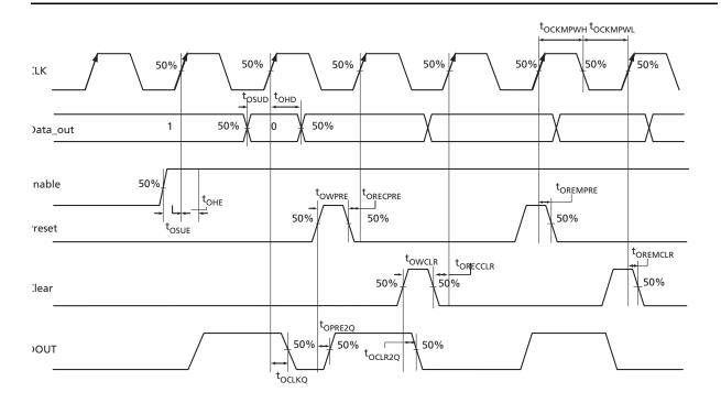
Figure 2-132 • Output Register Timing Diagram
