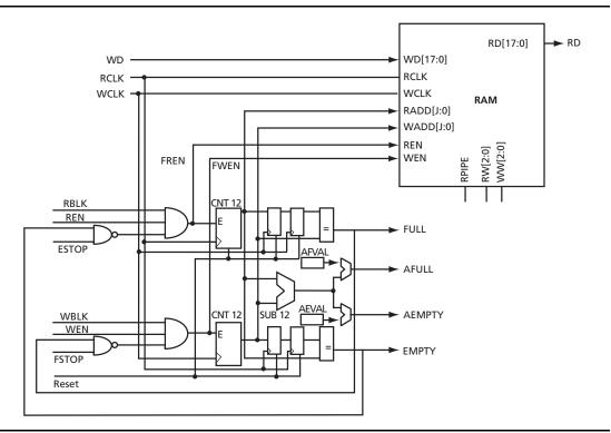
Figure 2-46 • Fusion RAM Block with Embedded FIFO Controller
