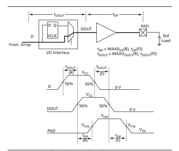
Figure 2-109 • Output Buffer Model and Delays (example)
