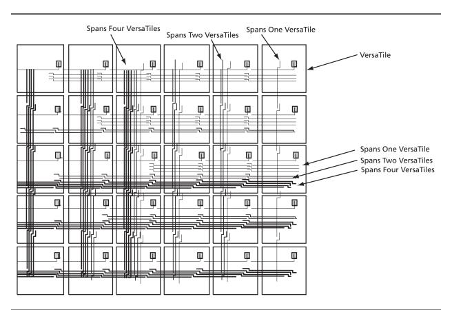
Figure 2-9 • Efficient Long-Line Resources
