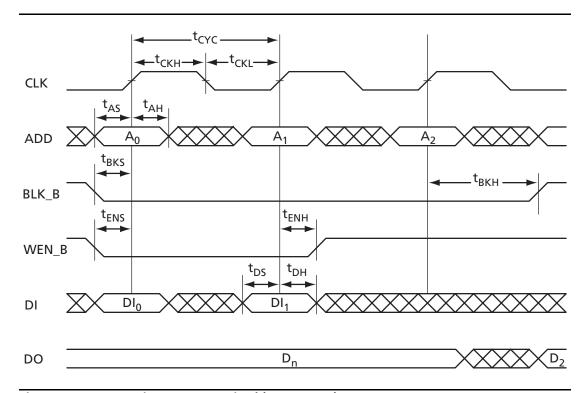
Figure 2-51 • RAM Write, Output Retained (WMODE = 0)
