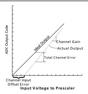
Figure 2-68 • Total Channel Error Example
