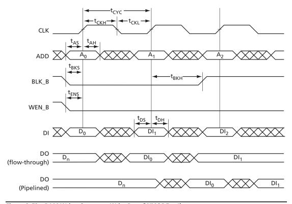
Figure 2-52 • RAM Write, Output as Write Data (WMODE = 1)
