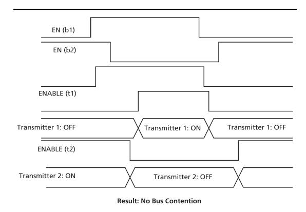
Figure 2-104 • Timing Diagram (with skew circuit selected)
