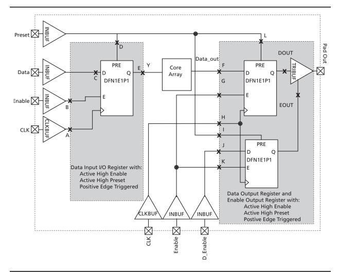
Figure 2-129 • Timing Model of Registered I/O Buffers with Synchronous Enable and Asynchronous Preset
