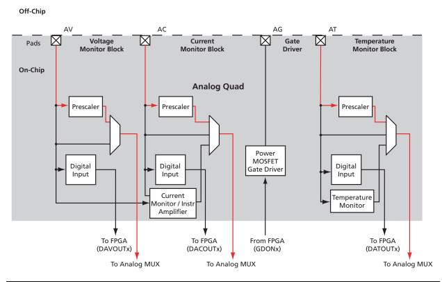
Figure 2-67 • Analog Quad Prescaler Input Configuration
