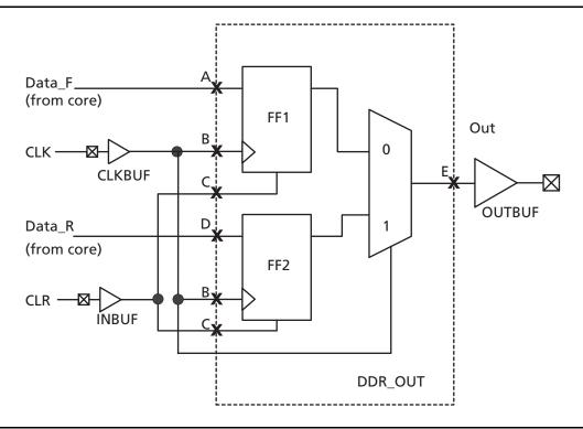
Figure 2-136 • Output DDR Timing Model
