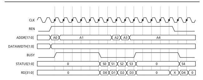
Figure 2-38 • Read Waveform (Pipe Mode, 32-bit access)
