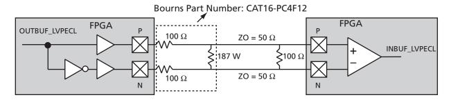
Figure 2-128 • LVPECL Circuit Diagram and Board-Level Implementation
