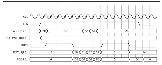
Figure 2-37 • Read Waveform (Non-Pipe Mode, 32-bit access)
