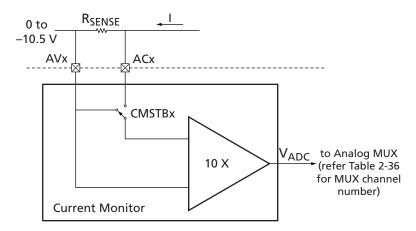
Figure 2-73 • Negative Current Monitor
