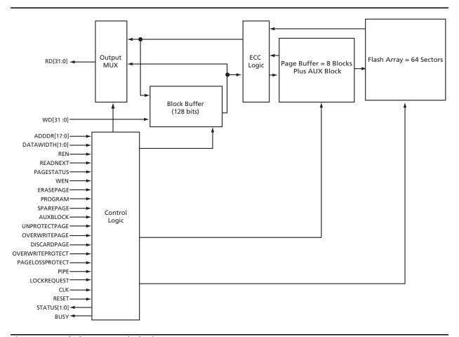
Figure 2-32 • Flash Memory Block Diagram
