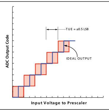
Figure 2-88 • Total Unadjusted Error (TUE)
