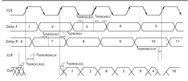
Figure 2-137 • Output DDR Timing Diagram
