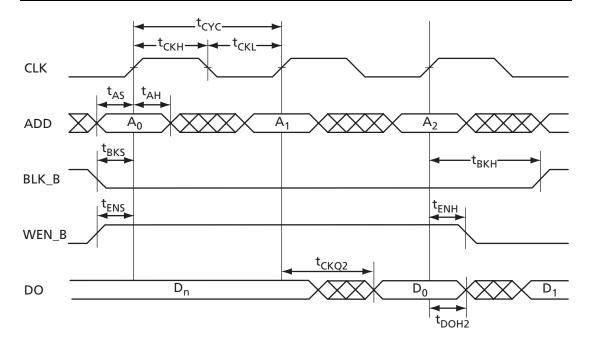
Figure 2-50 • RAM Read for Pipelined Output
