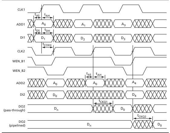
Figure 2-54 • Write Access After Write onto Same Address
