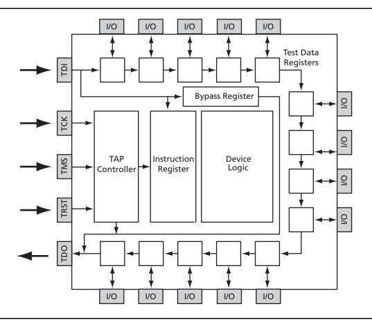
Figure 2-138 • Boundary Scan Chain in Fusion
