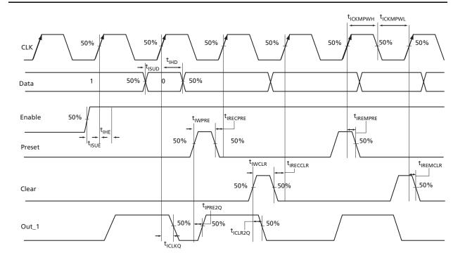
Figure 2-131 • Input Register Timing Diagram
