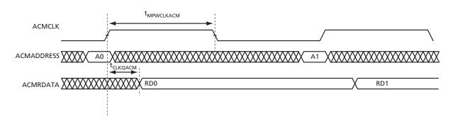
Figure 2-90 • ACM Read Waveform
