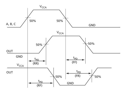
Figure 2-4 • Combinatorial Timing Model and Waveforms
