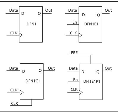
Figure 2-5 • Sample of Sequential Cells
