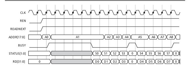
Figure 2-40 • Read Next WaveForm (Pipe Mode, 32-bit access)
