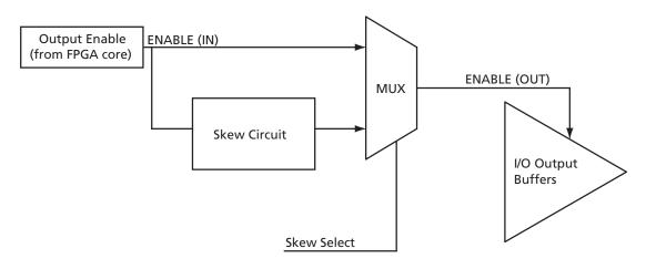
Figure 2-99 • Block Diagram of Output Enable Path
