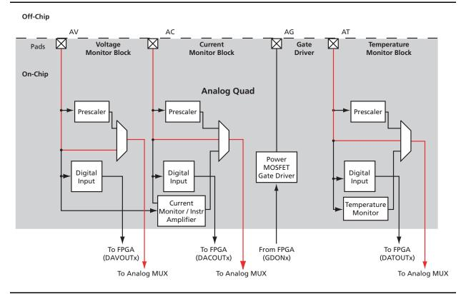
Figure 2-66 • Analog Quad Direct Connect
