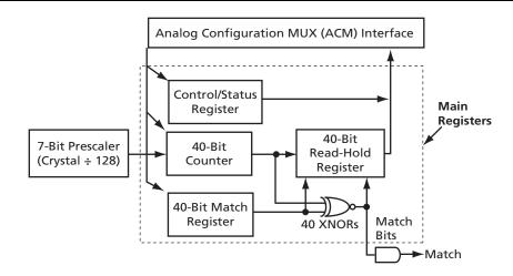
Figure 2-28 • RTC Block Diagram
