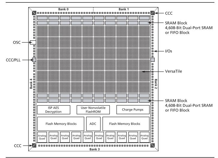
Figure 1-1 • Fusion Device Architecture Overview (AFS600)
