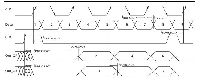
Figure 2-135 • Input DDR Timing Diagram
