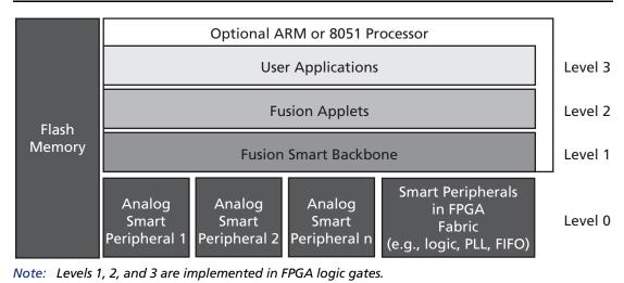
Figure 2-1 • Fusion Architecture Stack
