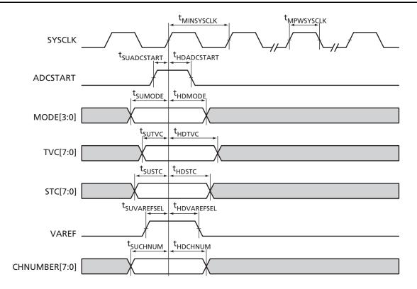
Figure 2-82 • Input Setup Time
