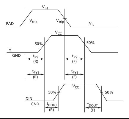
Figure 2-108 • Input Buffer Timing Model and Delays (example)
