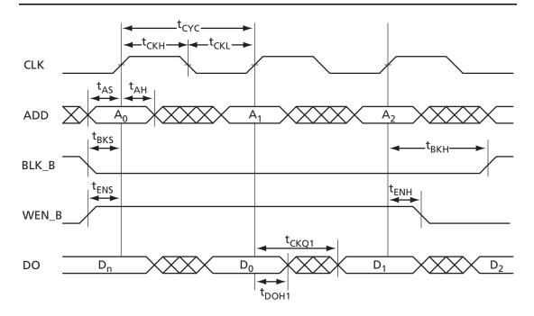
Figure 2-49 • RAM Read for Flow-Through Output
