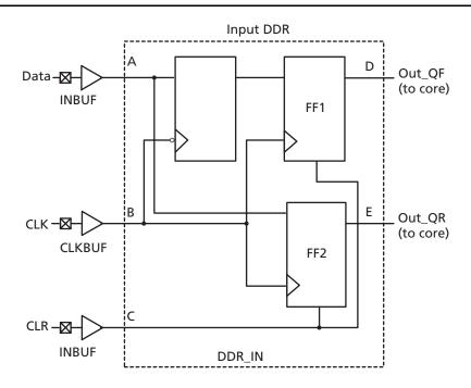
Figure 2-93 • DDR Input Register Support in Fusion Devices
