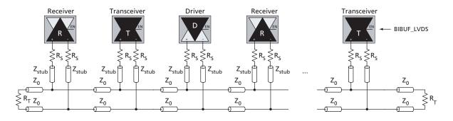
Figure 2-127 • BLVDS/M-LVDS Multipoint Application Using LVDS I/O Buffers
