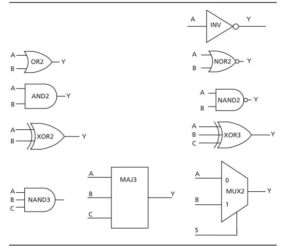
Figure 2-3 • Sample of Combinatorial Cells
