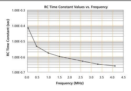
Figure 2-18 • Crystal Oscillator: RC Time Constant Values vs. Frequency (typical)
