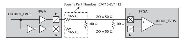
Figure 2-126 • LVDS Circuit Diagram and Board-Level Implementation
