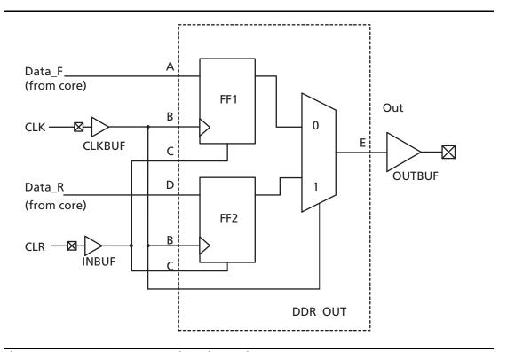
Figure 2-94 • DDR Output Support in Fusion Devices
