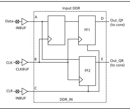
Figure 2-134 • Input DDR Timing Model
