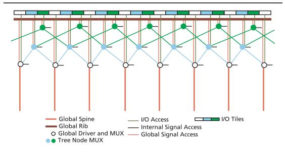
Figure 2-14 • Clock Aggregation Tree Architecture
