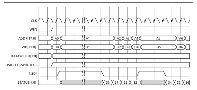
Figure 2-34 • FB Write Waveform
