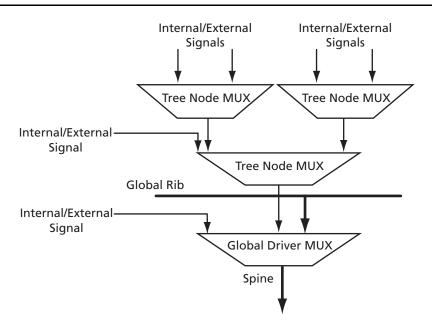
Figure 2-13 • Spine-Selection MUX of Global Tree
