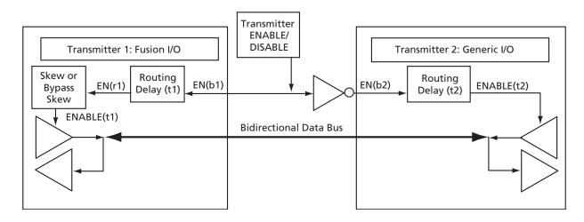
Figure 2-102 • Example of Implementation of Skew Circuits in Bidirectional Transmission Systems Using Fusion Devices
