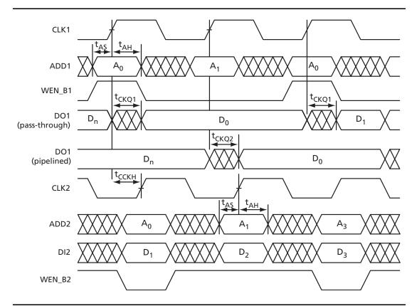
Figure 2-56 • Write Access After Read onto Same Address
