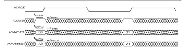
Figure 2-89 • ACM Write Waveform
