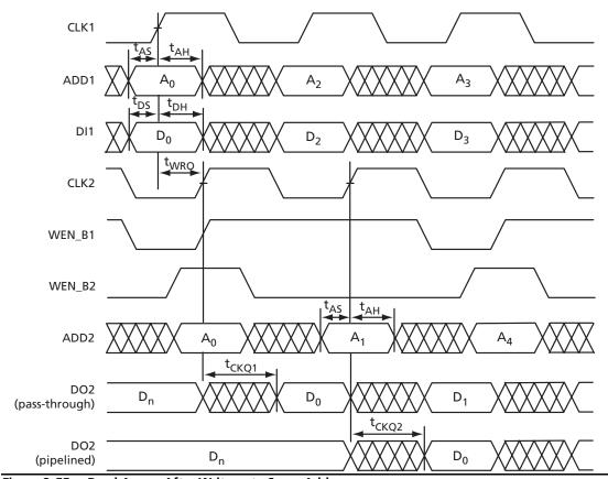
Figure 2-55 • Read Access After Write onto Same Address
