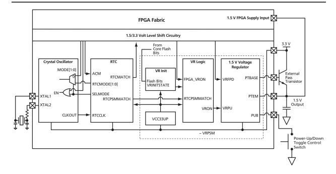
Figure 2-27 • Real-Time Counter System
