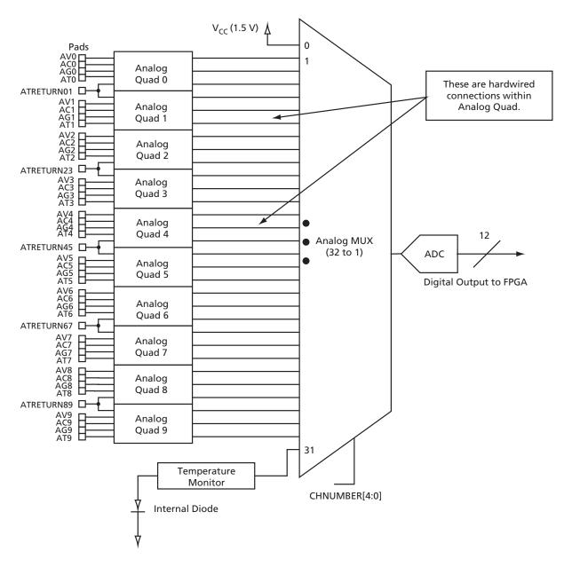
Figure 2-79 • ADC Block Diagram
