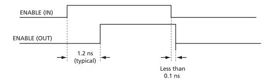
Figure 2-101 • Timing Diagram (option 2: enables skew circuit)
