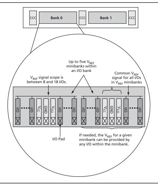
Figure 2-91 • Fusion Pro I/O Bank Detail Showing V<sub>REF</sub> Minibanks (north side of AFS600 and AFS1500)
