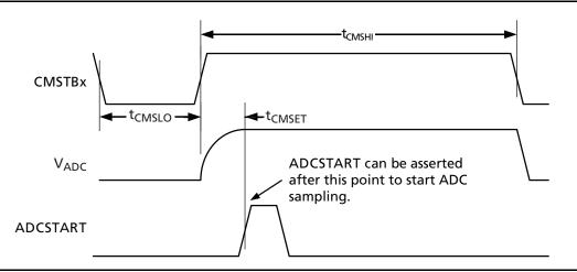
Figure 2-71 • Timing Diagram for Current Monitor Strobe
