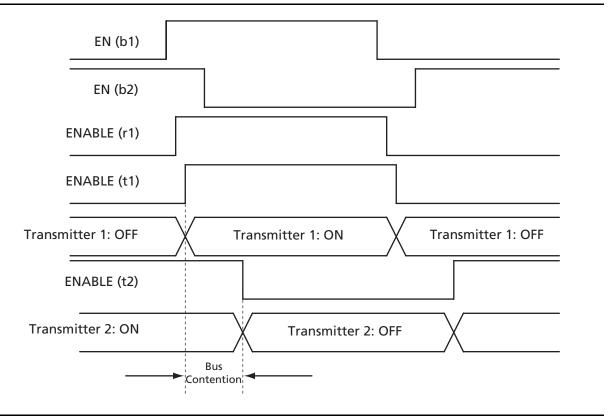
Figure 2-103 • Timing Diagram (bypasses skew circuit)
