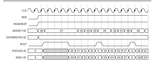
Figure 2-39 • Read Next Waveform (Non-Pipe Mode, 32-bit access)
