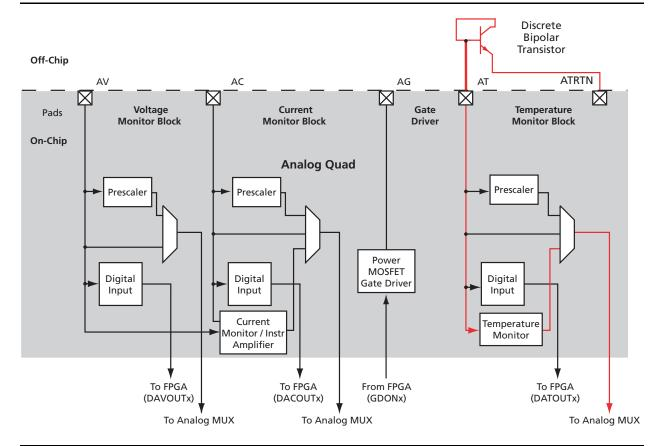
Figure 2-76 • Temperature Monitor Quad
