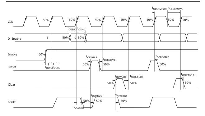
Figure 2-133 • Output Enable Register Timing Diagram
