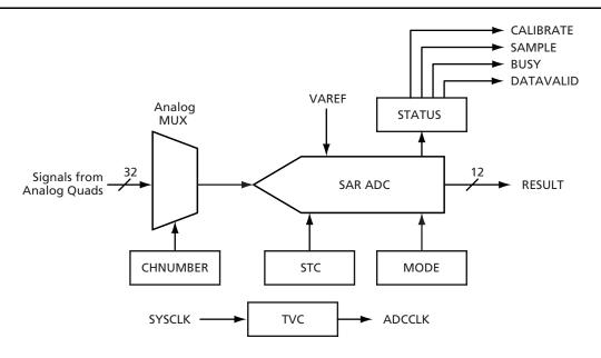
Figure 2-80 • ADC Simplified Block Diagram
