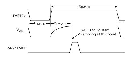
Figure 2-78 • Timing Diagram for the Temperature Monitor Strobe Signal
