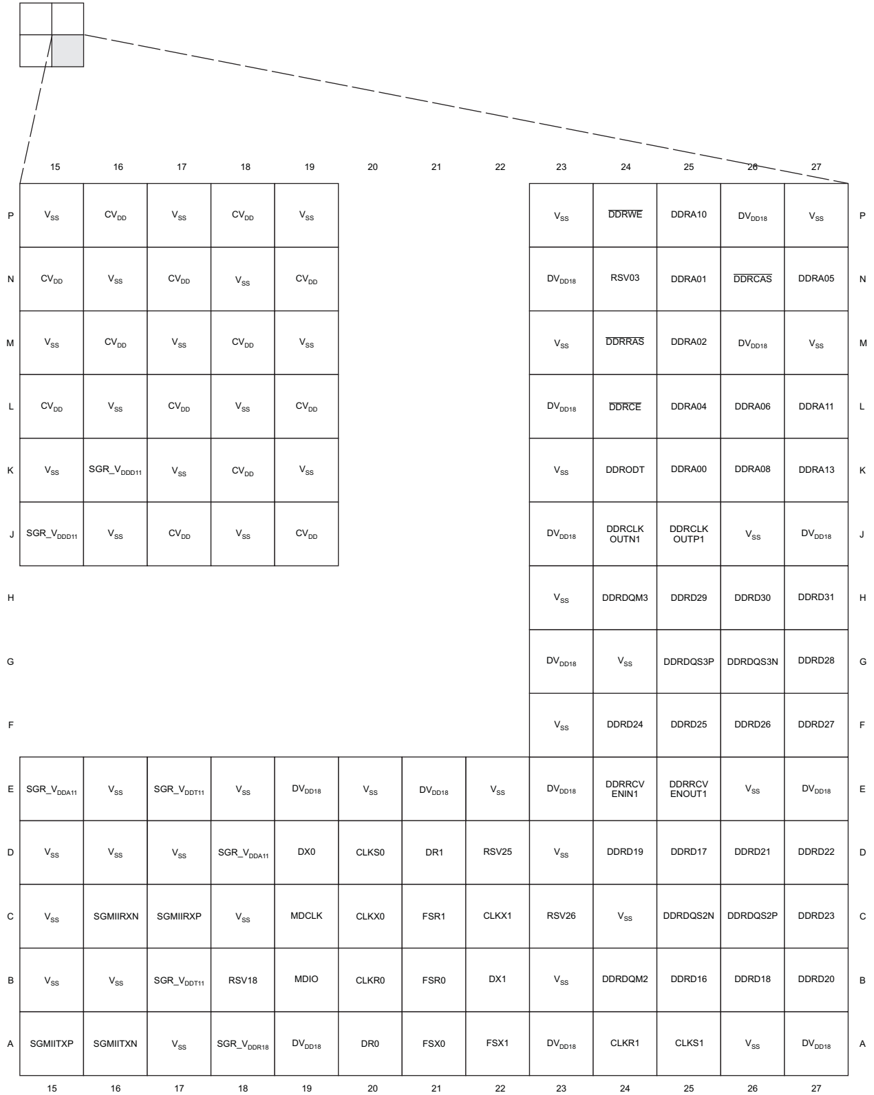
Figure 2-4. TCI6487/8 Pin Map (Bottom View) [Quadrant C]
