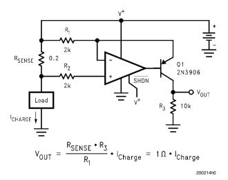
FIGURE 2. High Side Current Sensing
