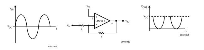
FIGURE 4. Half-Wave Rectifier with Negative-Going Output Referenced to V<sub>CC</sub>
