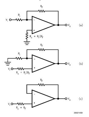
FIGURE 1. Canceling the Offset Voltage due to Input Bias
