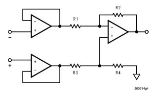
FIGURE 5. Rail-to-rail instrumentation amplifier
