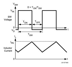
FIGURE 2. Typical Waveforms
