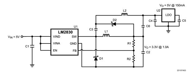
FIGURE 12. LM2830X (1.6MHz): Vin = 5V, Vo = 3.3V @ 1.0A & LP2986-5.0 @ 150mA
