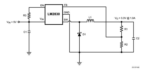
FIGURE 9. LM2830Z (3MHz): Vin = 5V, Vo = 3.3V @ 1.0A
