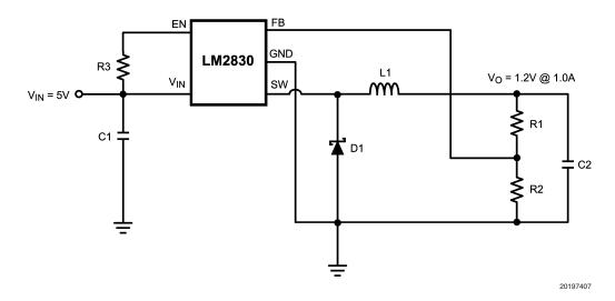
FIGURE 6. LM2830X (1.6MHz): Vin = 5V, Vo = 1.2V @ 1.0A
