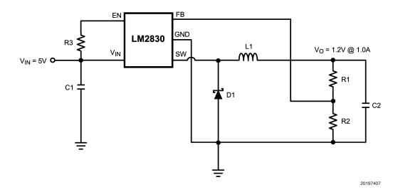
FIGURE 10. LM2830Z (3MHz): Vin = 5V, Vo = 1.2V @ 1.0A
