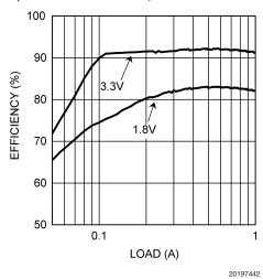
$\eta$  vs Load "X and Z" Vin = 3.3V, Vo = 1.8V
