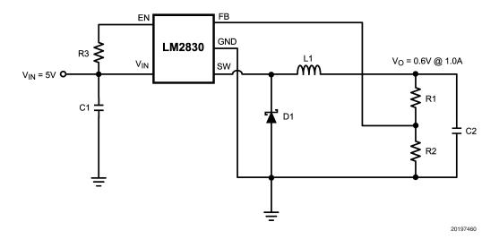
FIGURE 7. LM2830X (1.6MHz): Vin = 5V, Vo = 0.6V @ 1.0A
