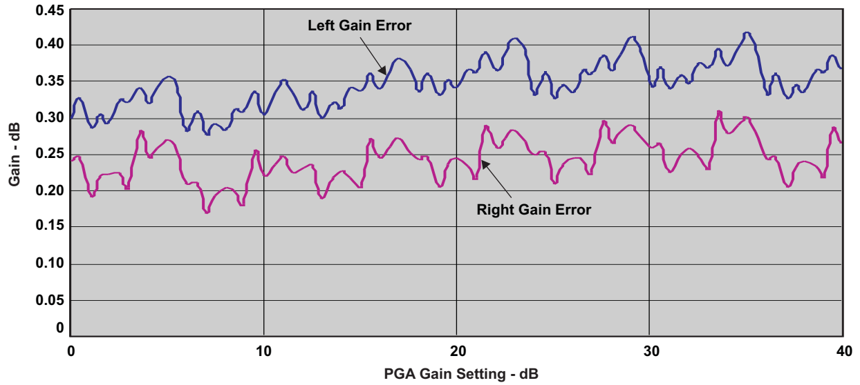
Figure 8. Single-Ended Gain Error
