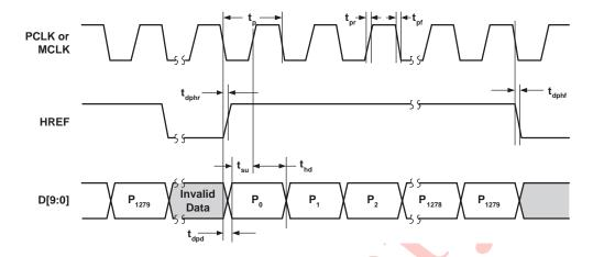
Figure 15 VGA Line/Pixel Output Timing
