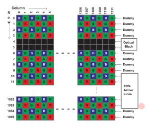
The color filters are Bayer pattern. The primary color BG/GR array is arranged in line-alternating fashion. Of the 1,359,232 pixels, 1,310,720 are active. The other pixels are used for black level calibration and interpolation.
