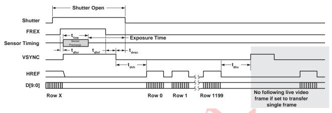
Figure 19 Frame Exposure Timing with EXPSTB Asserted
