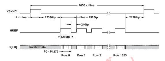
Figure 17 VGA Frame Timing
