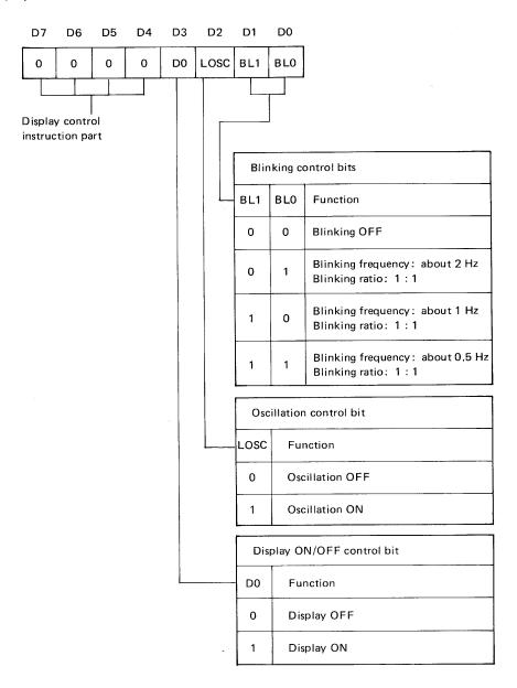
Note: The Display ON/OFF function is activated in synchronization with the Low-to-High transition of the  $\overline{H_{sync}}$  signal.
