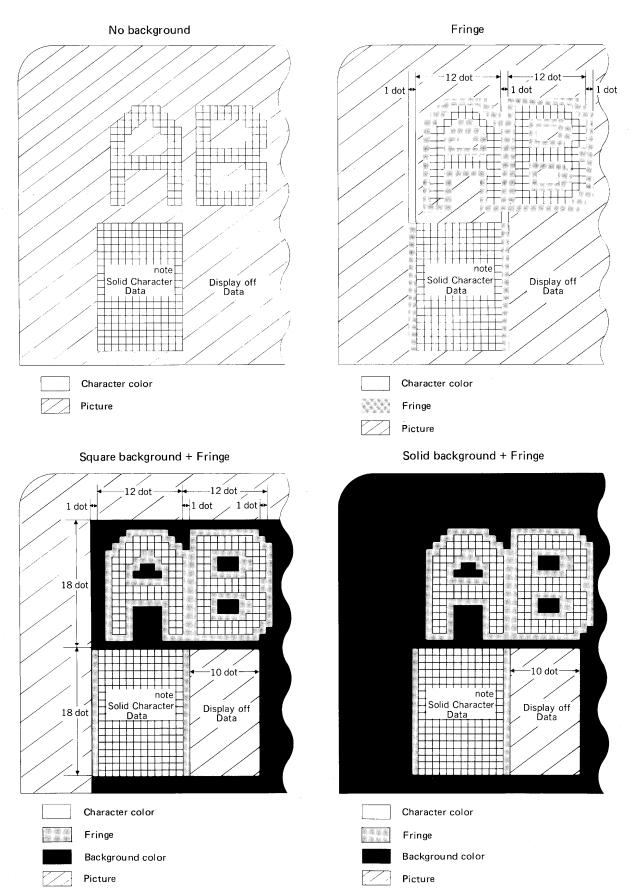
Note: The solid character data means the data of character code 1 F<sub>H</sub> (Standard type of NEC). It is possible to establish the background and the fringe at the same time.
