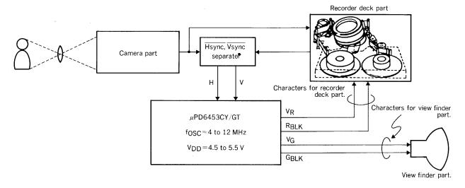
For example,  $V_G$  and  $G_{BLK}$  terminals are connected to the view finder part,  $V_R$  and  $R_{BLK}$  terminals are connected to the recorder deck part.
