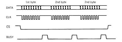
The internal data processing is performed on input of every one byte (8 bits). (See the paragraph "Recommended Timing" on page 17 for  $\overline{\text{CS}}$  and BUSY.)
