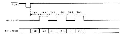
The leading and trailing edges of the mask pulse are synchronized with the trailing edge of HSYNC.
