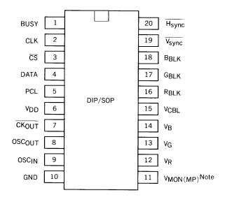
Note: Pin 10 (μPD6453CY/μPD6453GT) within parentheses is the mask code option to be used as the mask pulse. However, μPD6453CY-001/μPD6453GT-101 does not use the mask pulse, so pin 11 is used as monitor output V<sub>MON</sub>.
