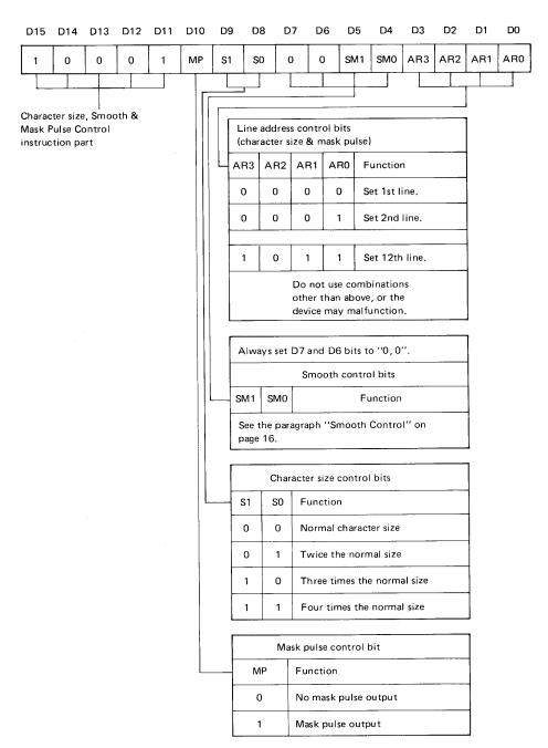
Note: The MP (mask pulse) control bit is valid only when the mask pulse function has been selected with the Mask code option. If this function has not been selected, set the MP bit to "0".
