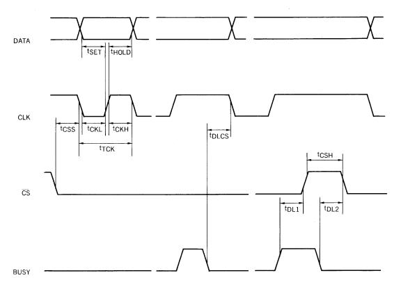
For format data, the BUSY signal goes low after the internal state is completely established. It also goes low when writing data into the VRAM is finished.
