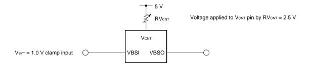
To input an external video signal with an amplitude of 2  $V_{P-P}$ , input a 1.0-V clamp signal to  $V_{SYT}$ , apply 5.0 V to the  $V_{CNT}$  pin, and set the amplitude of 2  $V_{P-P}$  by using the "output level control command".
