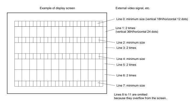
The size in the vertical direction (the number of horizontal scanning lines) is the size in field units.
