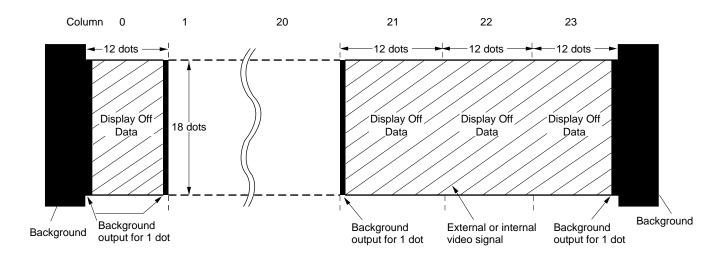
The background color is output on 1 dot on both the edges of Display Off Data when the Display Off Data is used.
