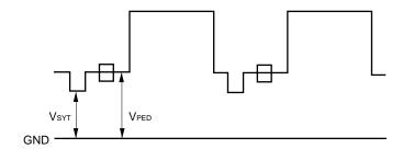
Match the level output from the VBSI pin in the external video signal mode with the level output from the same pin in the internal video signal mode.
