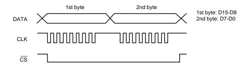
When transferring a 2-byte command, keep  $\overline{CS}$  low between the first byte and second byte.
