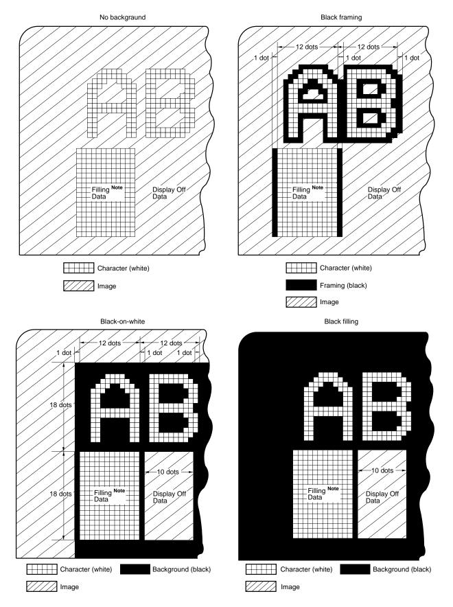
**Note** Filling data means  $1F_{H}$  ( $\mu$ PD6464A),  $6E_{H}$  ( $\mu$ PD6465) with the NEC's standard character.
