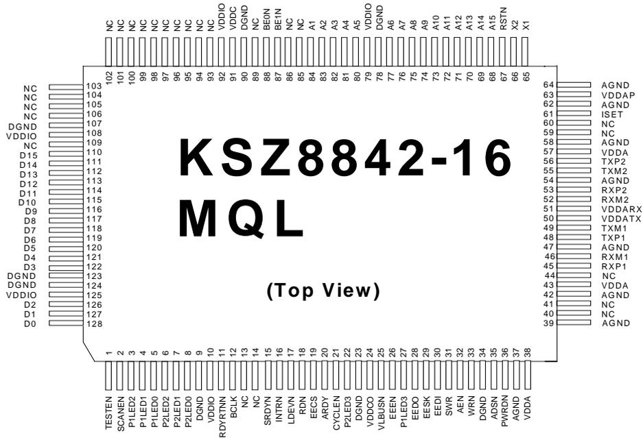
Figure 2. Standard – KSZ8842-16 MQL 128-Pin PQFP (Top View)
