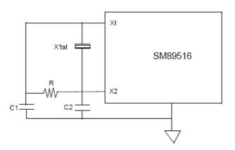
NOTE: Oscillation circuit may differs with different crystal or ceramic resonator in higher oscillation frequency which was due to each crystal or ceramic resonator has its own characteristics.
