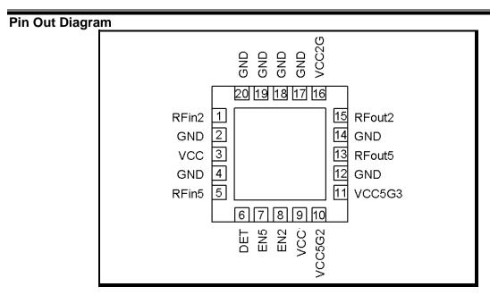
Figure 2: SE2580L Pin Out (Top View Through Package)
