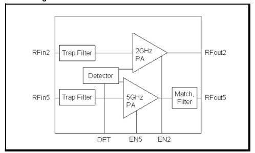
Figure 1: SE2580L Functional Block Diagram
