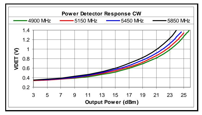
Figure 4: Preliminary SE2580L Power Detector vs. Output Power over Frequency into 1Mohm
