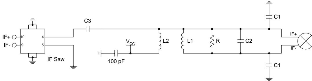
L1, C1, C2, and R form a current combiner which performs a differential to single-ended conversion at the IF frequency and sets the output impedance. In most cases, the resonance frequency is independent of R and can be set according to the following equation:
