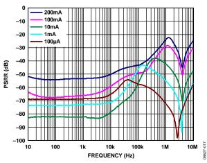
Figure 17. Power Supply Rejection Ratio vs. Frequency,  $V_{OUT} = 3.3 V$
