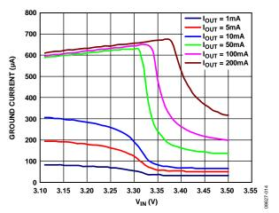
Figure 14. Ground Current vs. Input Voltage (in Dropout)
