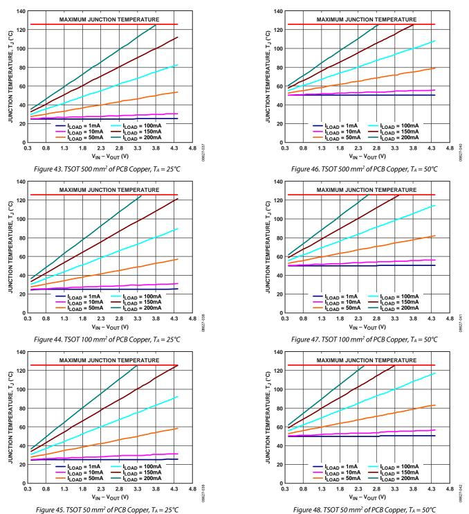
Figure 48. TSOT 50 mm<sup>2</sup> of PCB Copper,  $T_A = 50^{\circ}$ C
