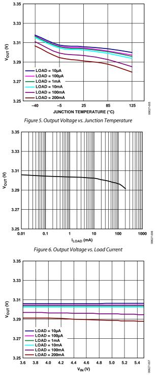
Figure 7. Output Voltage vs. Input Voltage
