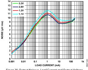
Figure 20. Output Noise vs. Load Current and Output Voltage,  $V_{IN} = 5 V$ ,  $C_{OUT} = 1 \mu F$
