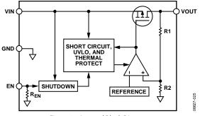
Figure 25. Internal Block Diagram
