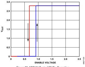
Figure 28. ADP151 Typical EN Pin Operation
