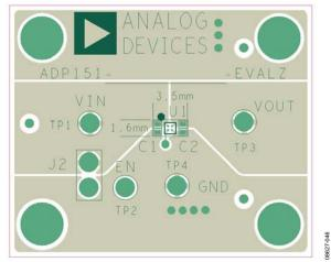
Figure 52. Example WLCSP PCB Layout
