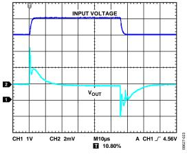
Figure 23. Line Transient Response,  $C_{IN}$ ,  $C_{OUT} = 1 \ \mu$ F,  $I_{LOAD} = 200 \ m$ A
