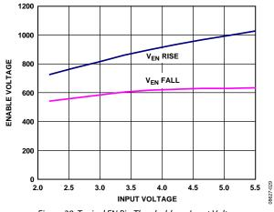
Figure 29. Typical EN Pin Thresholds vs. Input Voltage
