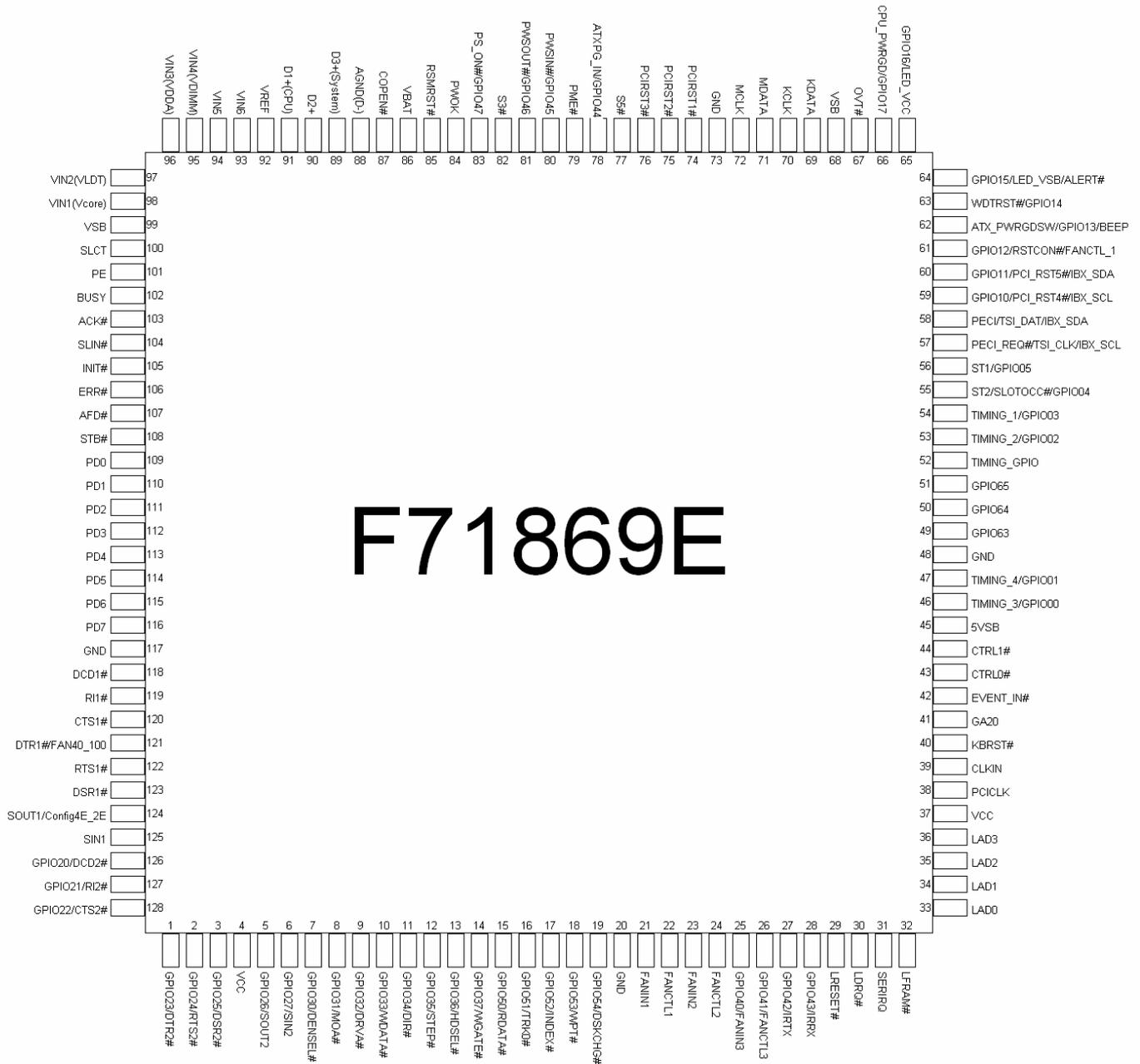
Figure1. F71869E pin configuration (14 \*14)
