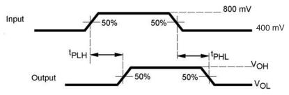
Figure 10. Propagation Delay
